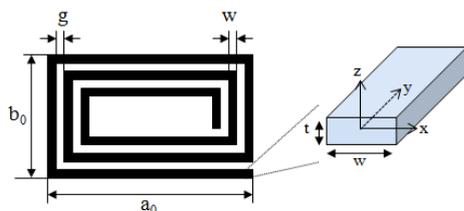
Figure 1. Top view (left) and cross-section (right) of a NFC antenna.
