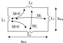
Figure 2. Partial and partial mutual inductances of a single-turn antenna
