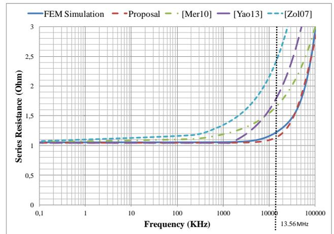
Figure 3. Series resistance  $R_s$  vs. frequency
